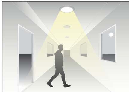
When motion is detected, sensor turns ON light.
