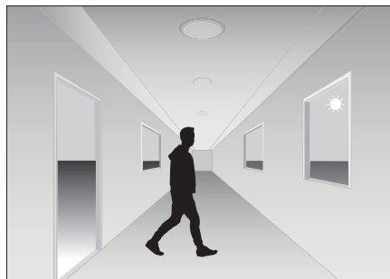
With sufficient daylight the sensor keeps the light OFF.
