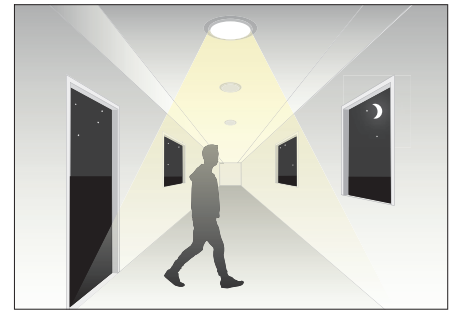
Light level goes up from standby dimming to 100% when motion is detected.
