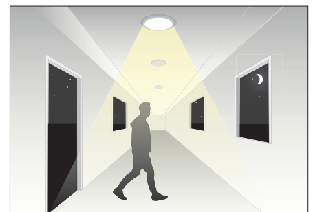
With insufficient daylight, the sensor turns light ON when motion is detected and OFF automatically after standby with no motion.
