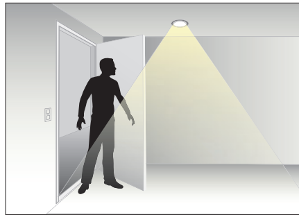
AUTO ON - Lights go on automatically when entering a room.
