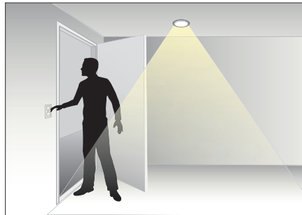
MANUAL ON - Lights have to be turned on manually when entering a room.
