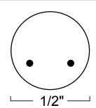
LED Rope Light: Cool White, Warm White and Blue lengths can be cut at 36" intervals. Red, Green and Yellow rolls can be cut at 54" intervals.
