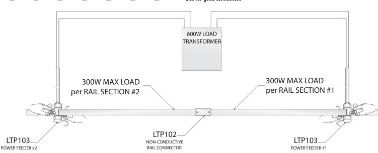
NOTE: 1.- USE NON-CONDUCTIVE (LP102) RAIL CONNECTOR TO JOIN RAIL SECTIONS,
