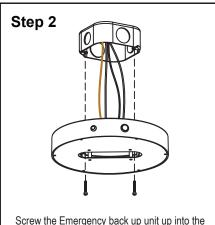
Screw the Emergency back up unit up into the junction box using the 2\*M4 screw provided,
