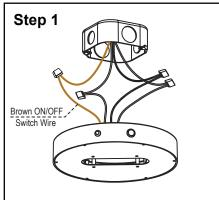
Connect the three cables available for connection into junction box. For Emergency back up unit, black wire is positive, white wire is negative, yellow wire is ground wire.
