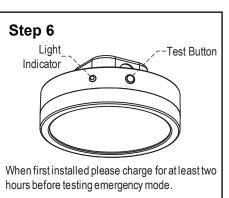
Press Button to enter EM mode, shown by the light indicator being off.
