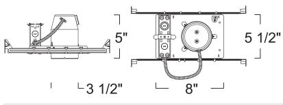
**Housing:** Pre-wired housing adjusts up to a 1 1/4'' ceiling thickness. Integral thermal protector to guard against improper lamping and installation. Trim is secured with torsion
