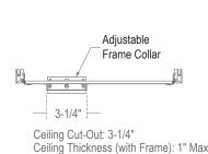
Trim is secured with torsion wing springs.
